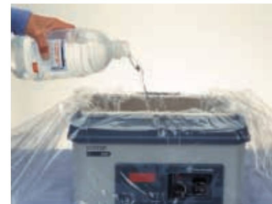
Figure 6 Sterile drape the water bath and fill with sterile water/saline, using a minimum of two liters. Turn ON and set temperature to 120°F (49°C).
