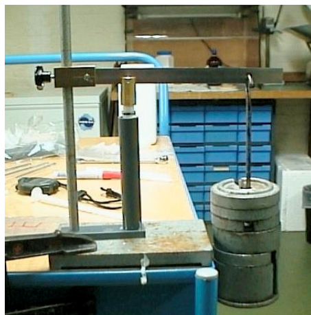
Fig. 5 Pressurizing bone cement
