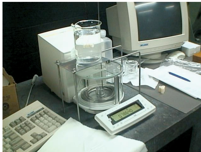
Fig. 6 The Archimedes test set-up
