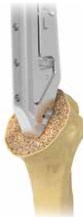
Figure C Broach Humeral Shaft
