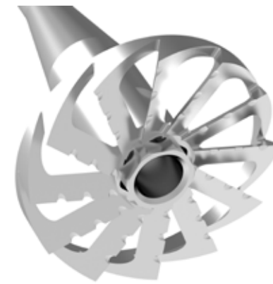
Figure 6 Improper Calcar Planer Assembly
